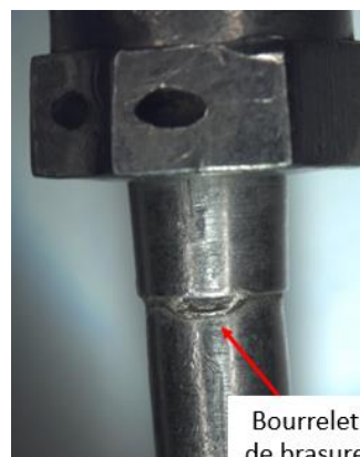
Figure 19 : bourrelet de brasure
