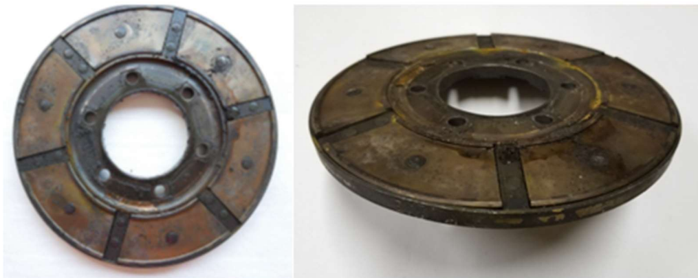
Figure 12 : plaque de retenue
