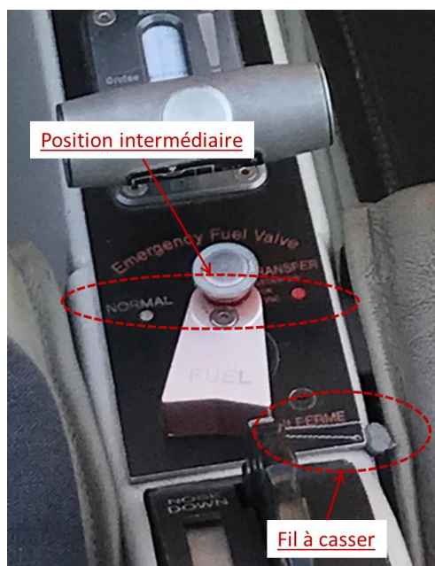
Figure 6 : commande secours carburant
