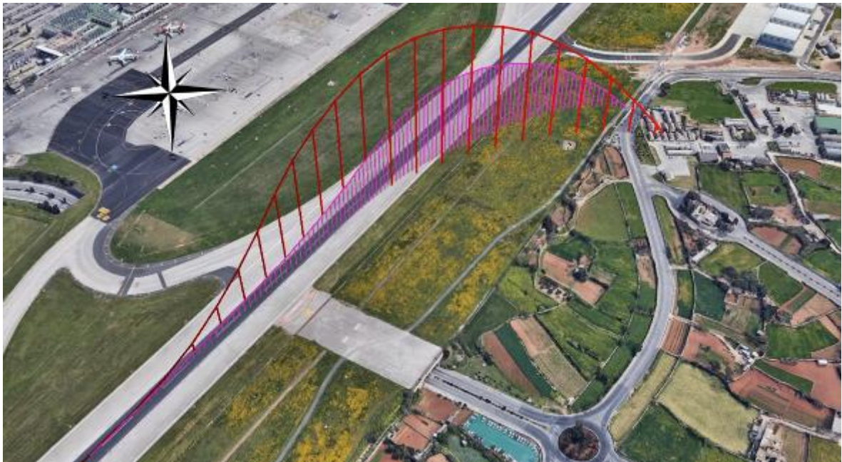
Figure 16: Comparison of the flight path of the PC7 (red) with that of the accident (magenta)
