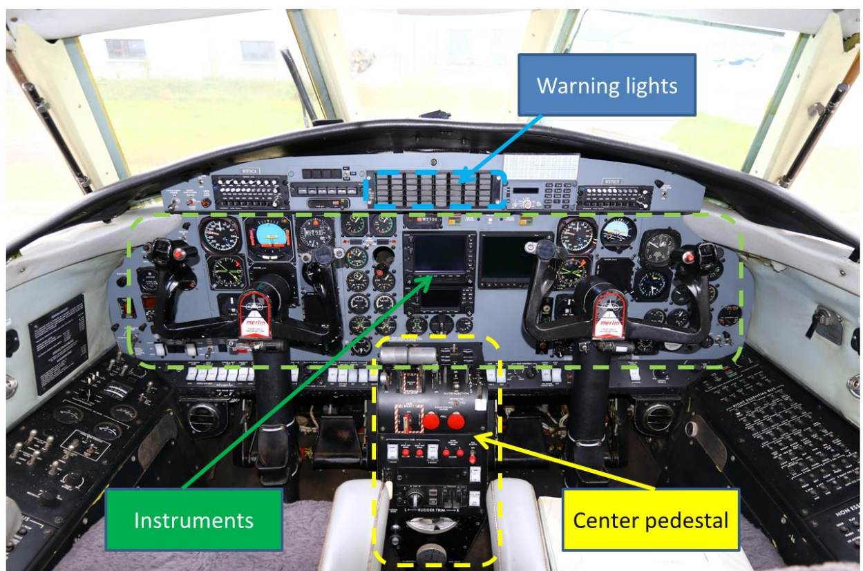
Figure 8: Illustration of the locations of the various cockpit elements submitted to examination
