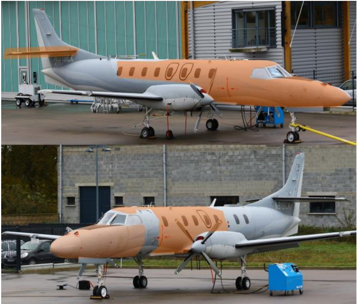
Figure 19: Illustration on the sistership of the missing parts or surfaces of the fuselage (marked in orange)
