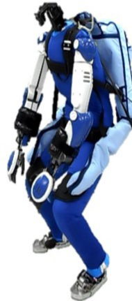
Fig.7 : Humanoid robot HRP-4 testing a wearable assistive device as a "subject" for a quantitative assessment.
