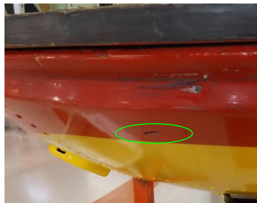
Perforation de la barque
