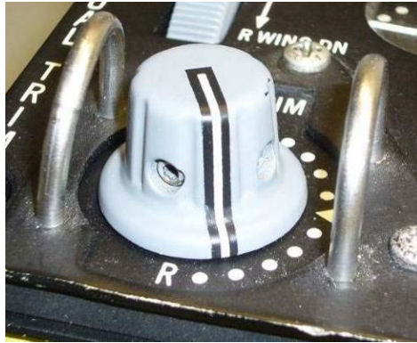
Picture D-3: Close view of Yaw Trim Knob and the two safety guards. Yaw trim knob of the figure is positioned to -8^{\circ} (8 degrees to the right). Every dot corresponds to 2 degrees.
