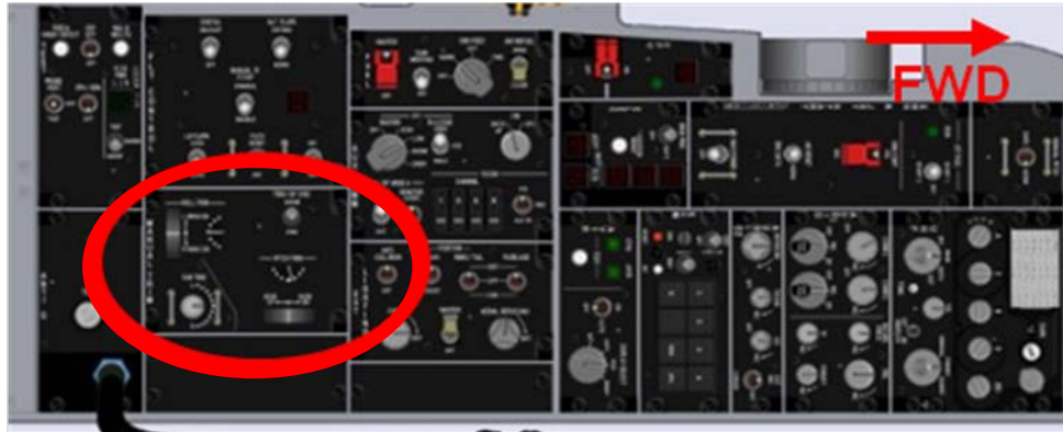
Figure D-1: F-16 Left Console with Manual Trim Panel (For reference only)
