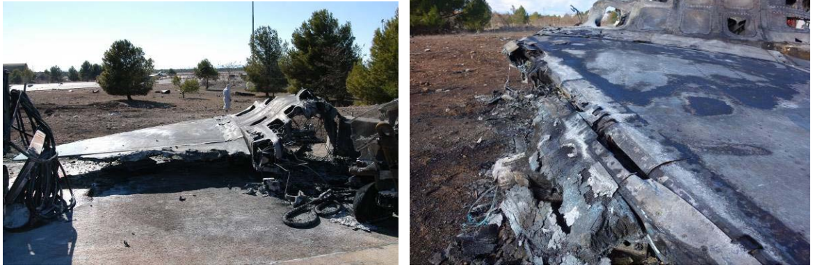
Pictures B-17: The LH wing (rear view) and close view of LH Leading Edge Flap
