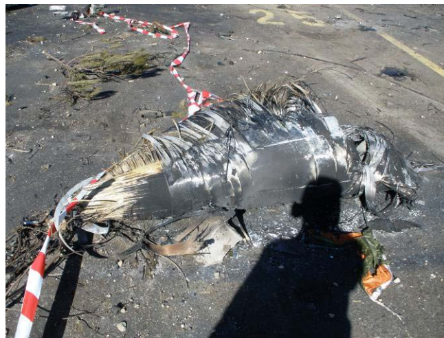
Picture B-11: The radome totally destroyed
