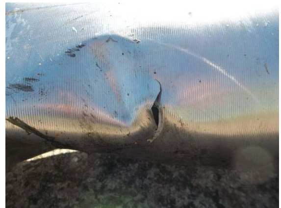
Pictures B-22: Close view of the fracture of the case of hydrazine tank. Hydrazine had been leaked from that point.
