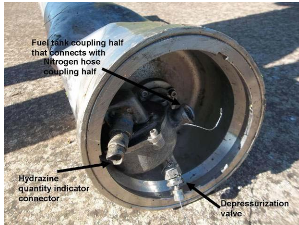
Picture B-23: Damages on FWD section of hydrazine tank.
