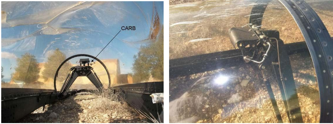
Pictures B-8: Canopy Release Bolt (CARB) properly operated
