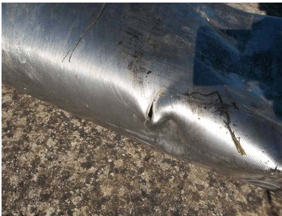
Pictures B-22: Close view of the fracture of the case of hydrazine tank. Hydrazine had been leaked from that point.
