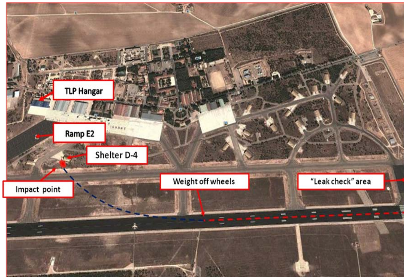
Picture B-1.: View of the Albacete AFB with the main runway, facilities and the MA trajectory (approximate). With red line is the MA trajectory before it becomes airborne and with blue afterwards
