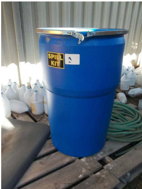
Pictures B-25: Hydrazine contaminated soil collected in special spill kit and hydrazine tank was stored in adequate salvage drum. Due to hydrazine tank's deformation it could not be installed in its appropriate container.
