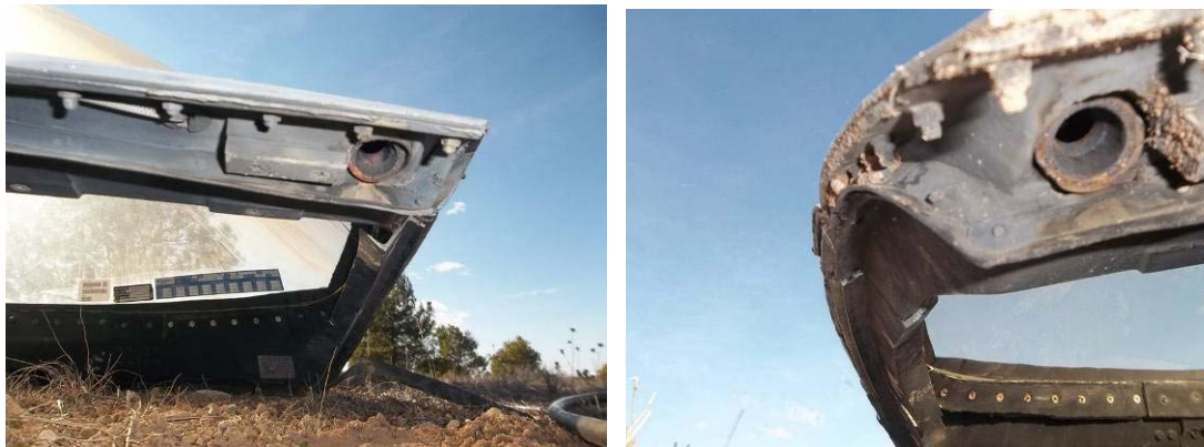
Pictures B-9: Canopy Remover Assemblies properly operated
