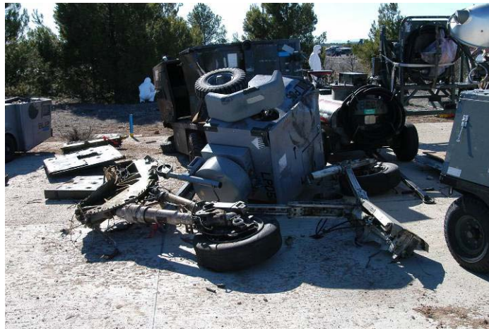
Picture B-18: MLG and drifted ground equipment
