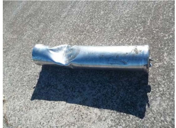
Pictures B-21: View of hydrazine tank's distortion (All Hydrazine tank pictures have been taken in Greece and not at crash site)
