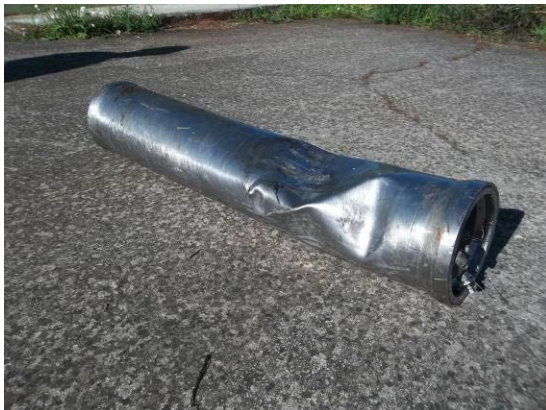
Pictures B-21: View of hydrazine tank's distortion (All Hydrazine tank pictures have been taken in Greece and not at crash site)
