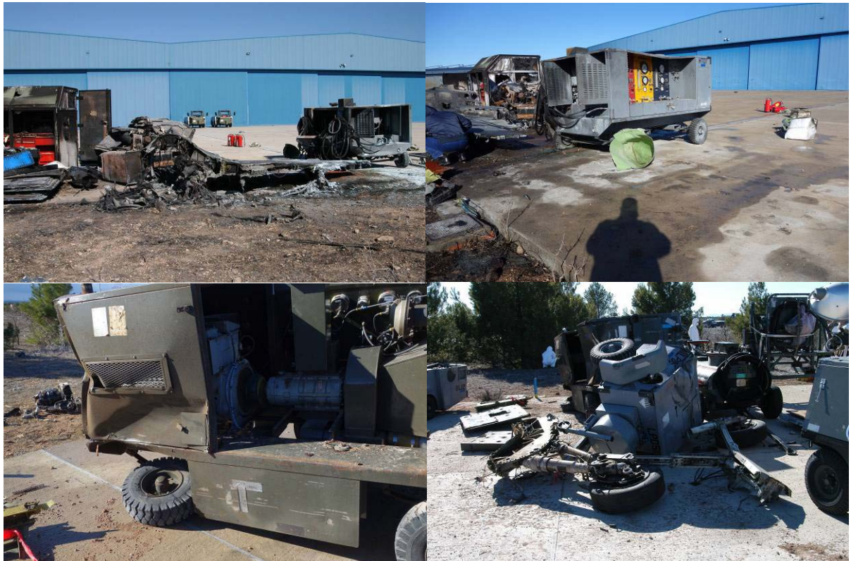
Pictures 34: Damages caused by MA's pieces on ground equipment
