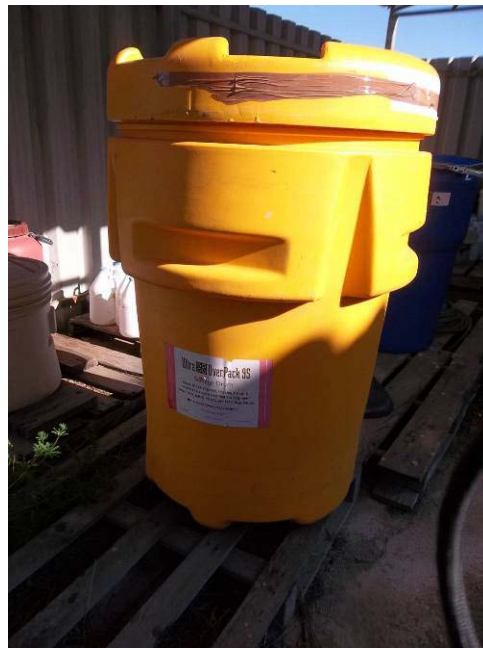
Pictures B-25: Hydrazine contaminated soil collected in special spill kit and hydrazine tank was stored in adequate salvage drum. Due to hydrazine tank's deformation it could not be installed in its appropriate container.
